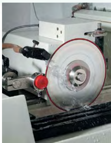
Preparation for the analysis of the SPR-joint.
