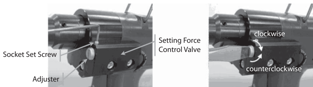
Figure 14: Adjustment of Setting Force
