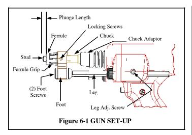
loosened, the foot will move freely in all directions. Adjust the foot so that the stud is centered in the ferrule and no contact occurs between the stud and the ferrule during retraction or forward plunge of the stud. Tighten the locking screws after centering the stud.
