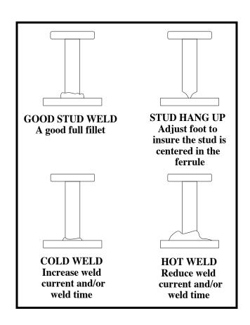
Figure 7-1 WELD INSPECTION
