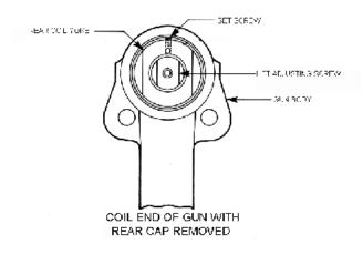
Figure 6-2 LIFT ADJUSTMENT
