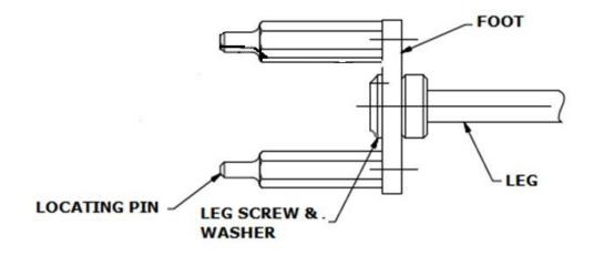
Figure 3.3b Tripod Foot & Leg Assembly
