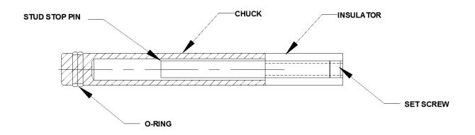
Figure 8.1 Stud Stop Pin Assembly
