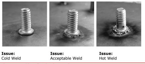
Figure 7.1 Weld Quality Visual Inspection
