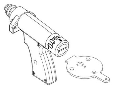
Figure 4.3 Contact Gun with NCD+ Set-Up Tool #525-001-200
