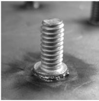
Issue: Acceptable Weld Weld Flash: Normal, No significant weld splatter Weld: Good, strong Adjustments: None required
