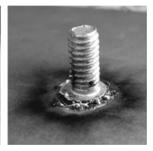
Issue: Too Hot Weld Flash: Excessive flash and weld splatter Weld: Weak, May break Adjustments: Reduce voltage, increase spring pressure, or reduce capacitance
