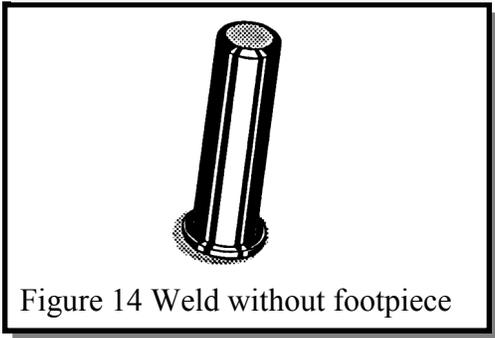
Figure 14 Weld without footpiece
