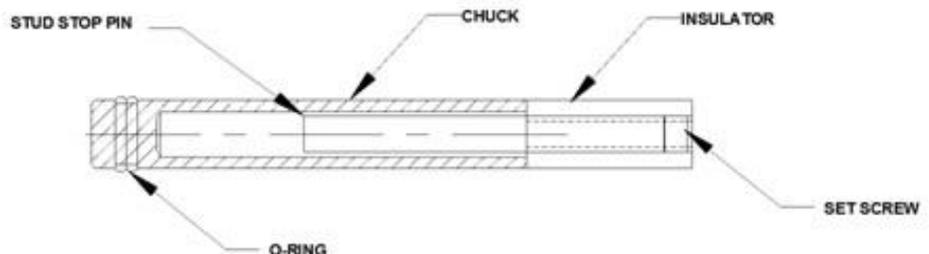
Figure 3.1 Chuck and Stop Assembly
