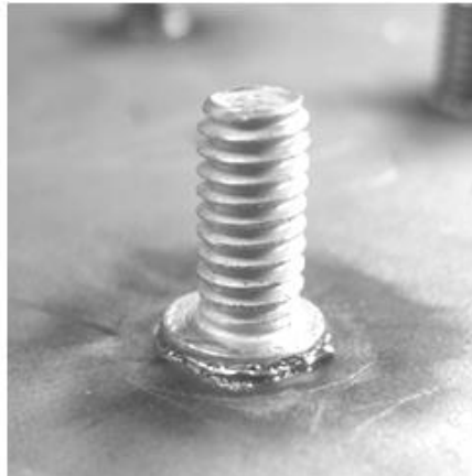
Situation: Acceptable Weld
