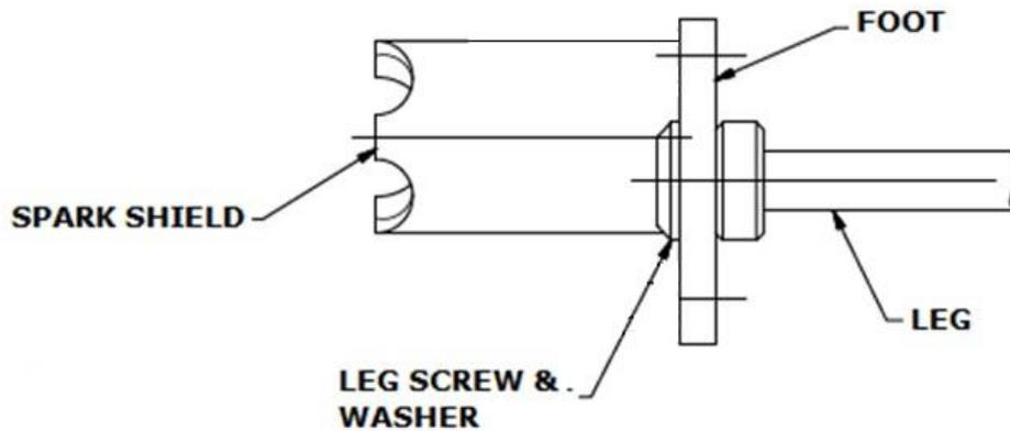
**Figure 3.2a Spark shield Foot & Leg Assembly**
