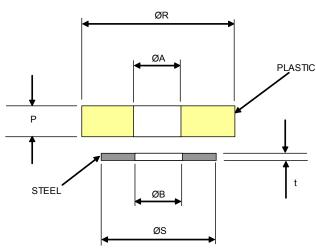
ØA = 6.8mm DRILLED ØB = 6.8mm PUNCHED
