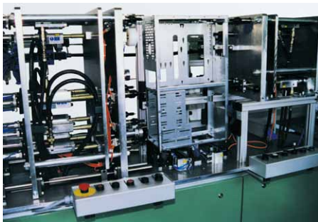
Hydra 1000 offers e.g. for complete assembly of computer chassis
