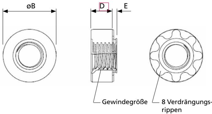
Material: Stahl ASTM A 583 M
