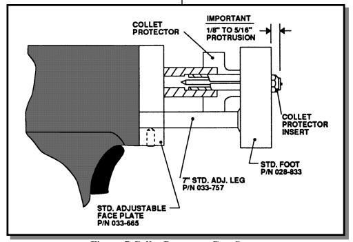
**Figure 7 Collet Protector Gun Setup**
