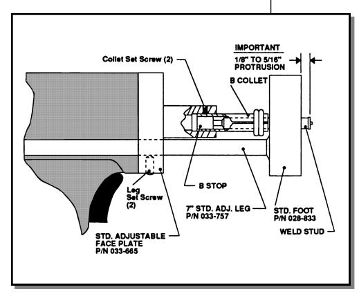
Figure 6 Standard Gun Setup
