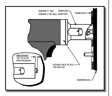
Figure 8 Template Adapter gun setup
