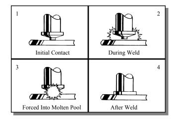
(FIGURE 1 CONTACT CD WELD)
