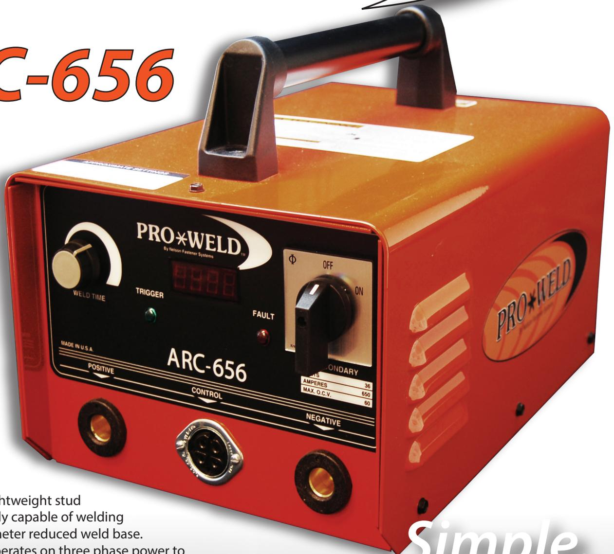
This is a compact, lightweight stud welding power supply capable of welding studs up to 1/2" diameter reduced weld base. The power supply operates on three phase power to produce a smooth, stable welding arc. The front panel digital display indicates the weld time, which is infinitely adjustable for precision and repeatability.
