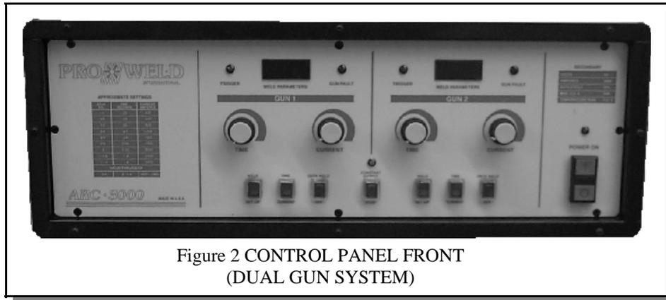
Figure 2 CONTROL PANEL FRONT
