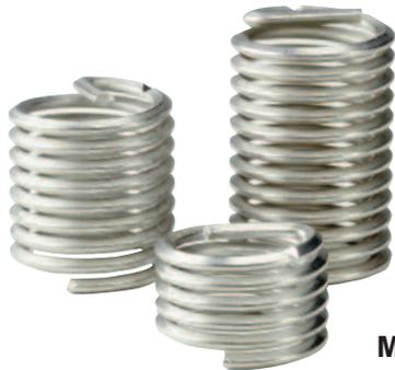
Heli-Coil repairs are available in the following standard thread series and size ranges: **Inch Coarse** (#8 thru 1-1/2), **Inch Fine** (#10 thru 1-1/2), **Metric Coarse** (M3 thru M20), **Metric Fine** (M8 thru M18), **Spark Plug** (10mm, 12mm, 14mm, 18mm & 7/8"), and **Pipe Thread** (1/8" thru 1").
