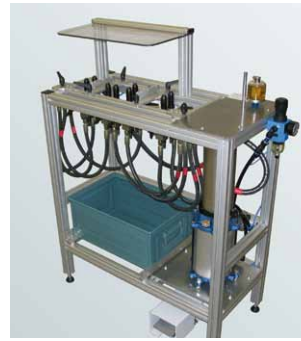
8-head station with adjustable rivet modules for the assembly of transformer and starter to base plate of fluorescent lamp
