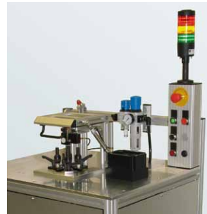
Adjustable 4-head MAS assembles two types of seat belt retractors; on two positions modules are adjustable against stopper
