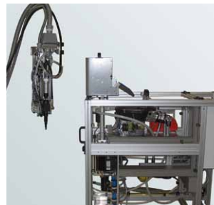
The unit consists of placing head and supply unit with integrated control unit
