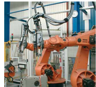
Autosert® placing head mounted on robot arm
