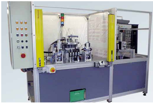
Multiple riveting with automatic rivet feed and process monitoring
