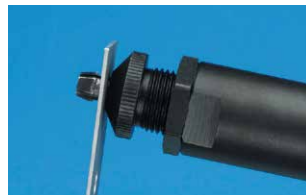
Insert the punch (fixed onto the 74290 tool) into the round hole
